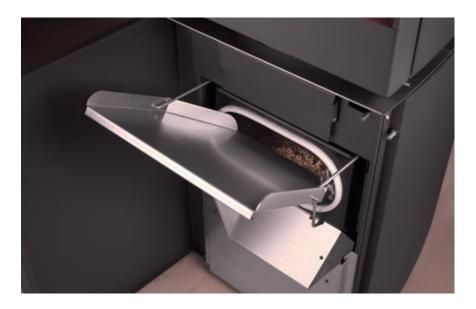
The loading hatch enables pellets to be loaded at hip height. The hopper can hold 18kg, corresponding to 10 hours of heating at maximum power, 30 hours of heating at minimum power. The ash pan allows for easy removal of ash. The design of the appliance makes glass cleaning and maintenance simple.
